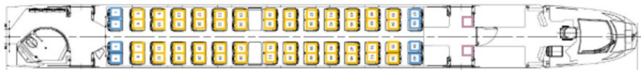
DPTS Coach E—835 Car 5 60 standard seats, 8 of which are priority, 2 additional tip-up seats making 62 in total
