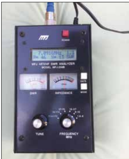
Fig. 4: Measured SWR and impedance on the 40m band.
