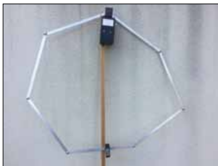
Fig. 5: The 10/12m loop with remote tuning box.
