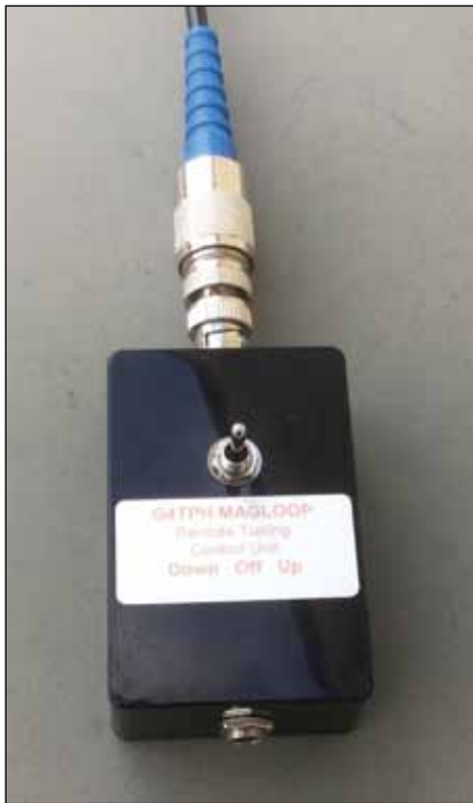
Fig. 7: The switch box as used at the shack end.
