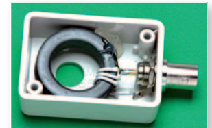
Fig. 3: The unusual method of coupling into the loop winding.
