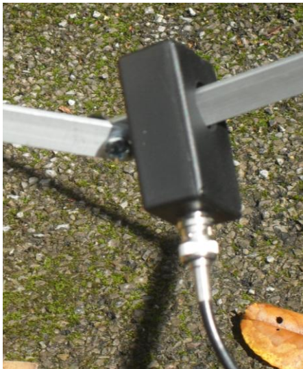
Mk 2 Load unit with cable attached
