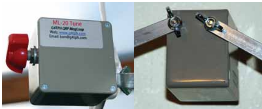
PHOTO 5 & 6: The tuning unit is fitted to the two open end of the loop.
