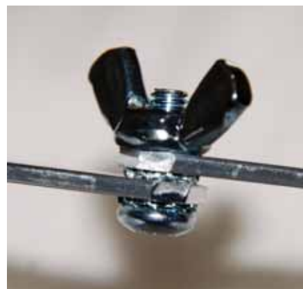
PHOTO 7: Shake proof washers were fitted between the bars.
