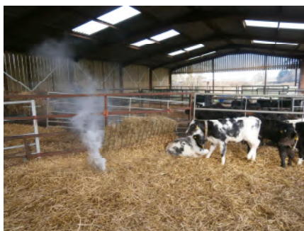
Smoke testing a calf shed
