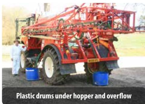
Plastic drums under hopper and overflow
