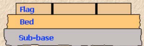
Regular thickness of wet-press flags makes screed bedding possible
