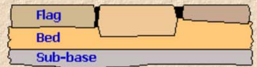
Random thickness of natural stone flags makes screed bedding impractical
