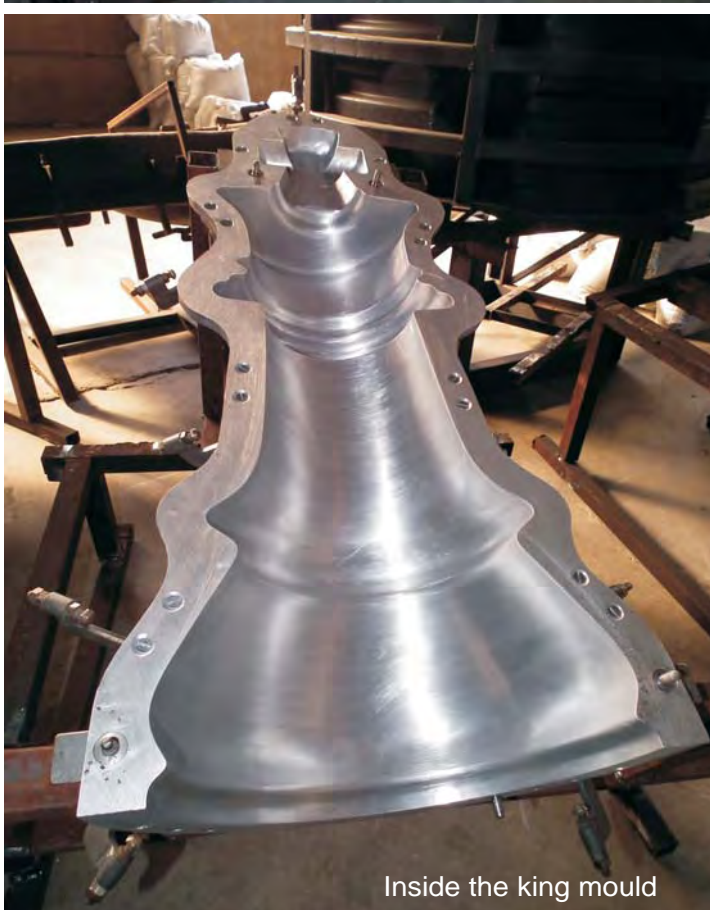
King aluminium roto-moulding assembly
