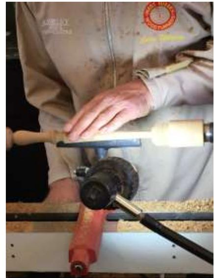
Once the handle and the stem have been turned down to size and happy with the finish on the handle. Time to reset the wood to an offset, which have been previously drilled in the ends of the spindle and made sure the screw chuck fits in. This is to make sure that the screw chuck does not split the wood when repositioning your already half turned item.
