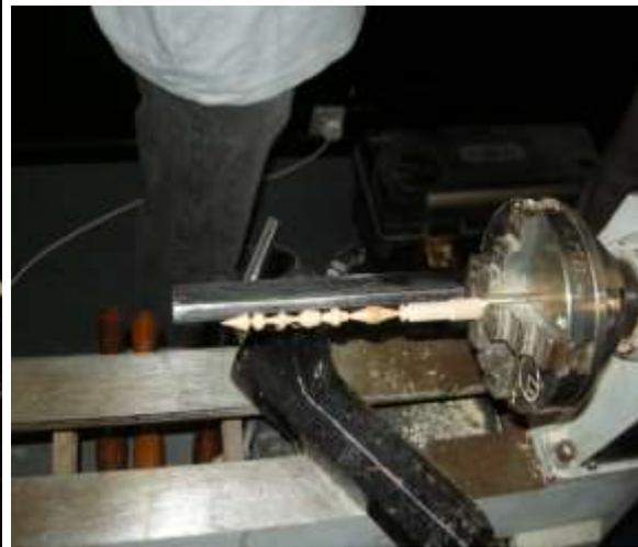
Gary uses a home-made steady to stop the finial flexing whilst he turns it.
