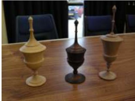
Les uses a hollow live centre. If you don't have one you can make your own. He made a mould for the finial end from wet paper towel. He then removed the base from the chuck and put the top back into the chuck with the finial actually inside the chuck so he could turn the inside of the top. He removed the waste.
