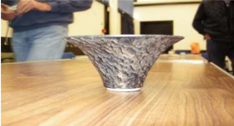
To texture the bowl he used a Sabretooth Burr on a Dremel. Do not use the fine ones if you want a decent texture. Les then introduced his blow torch going over the bowl to remove any rough and fuzzy bits on the surface. He used the sanding wheel again to smooth down the surface. He then applied sealer and sprayed with black lacquer. If the surface still feels rough, as sealer can raise the grain, sand it down again. He then dry brushed the surface with Gold Gilt Cream.
