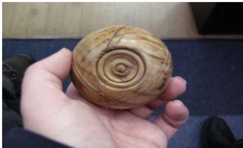
As a quick demonstration Jason put a blank between two ring centres. He used a ¼ inch bowl gouge to turn a mushroom. In order to under cut the mushroom he simply reversed the piece to make it more comfortable. To finish you can sand down the top and the base using a disc sander or a sanding arbour in the head stock.
