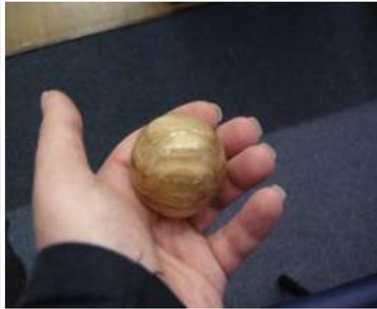
Jason then turned a third ball. This time he cut some lines into it. At home he would have used a burn wire to burn the lines. He placed the ball into a hollow wooden tube which he placed in the chuck. He put a flat on the ball and drilled a hole using a Forstner bit to take a small clock mechanism. Always drill holes slowly. He turned the ball in the tube and put another flat on so the clock would not roll around. He finished the bottom with some beads.
