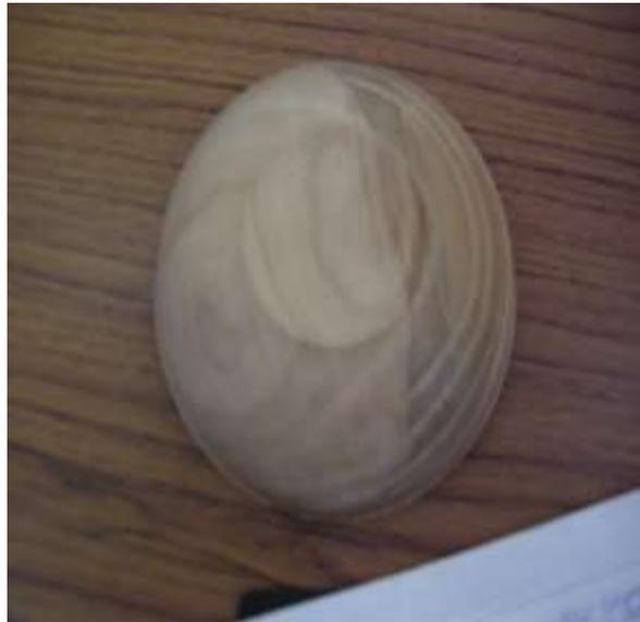
Next Keith showed us how he turned an Off centre bowl using the larger Doughnut chuck. To enable him to be able to work with the chuck Keith used a Morse taper extension.
