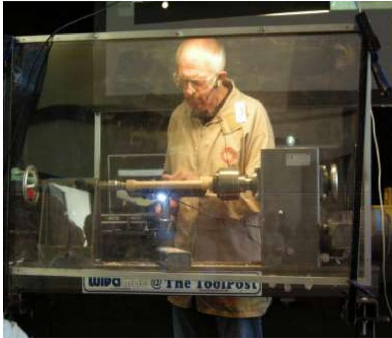
The first project was to be a letter opener. I have put one set of instruction as an extra page. He was using Beech. Colin says to make any marks across the grain. Ensure you leave a square on each end. Colin uses a home made screw chuck for one end of the Opener and an Axminster centre for the tail stock end. The Axminster comes with a variety of tips and costs approximately £62 (before getting Club discount).
