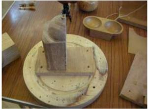
Basically you make a face plate Then you make another jig comprising a flat piece to which is attached an upright piece. (that's the bit with what looks like a partially turned bowl on the top of it). Gary screws these together. The blank you intend to make into your double bowl is then screwed onto the upright in such a way that the two screw holes are in the part that you will hollow out to give you the bowls.
