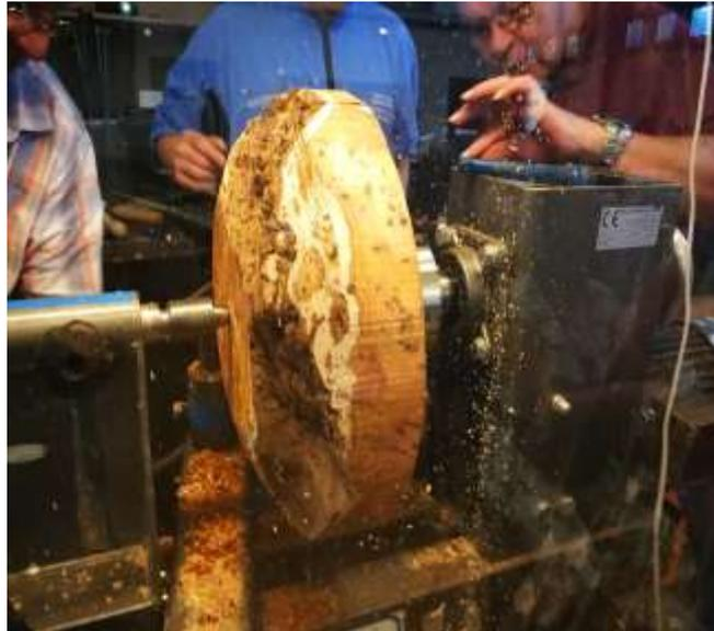
Mark started working from the headstock towards the base. The reason for doing this is that by doing a push cut from the base he would risk losing the top of the bowl.
