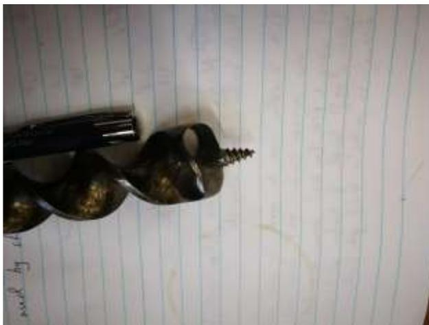
This is a Bull nose drill to help drill into End grain. Normal bits will tend to shred the wood rather than cut a nice clean hole.
