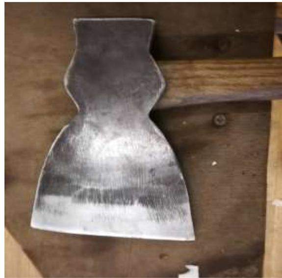
This is a side axe, which only has a bevel on one side and the handle is slightly offset to avoid damage to your knuckles.
