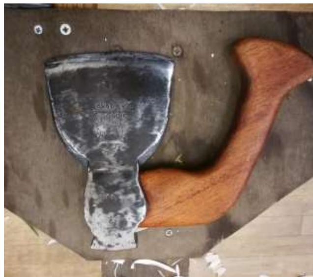
The handle of this axe is designed so that you do not have to keep bending your wrist thus avoiding Repetitive Strain Injury.
