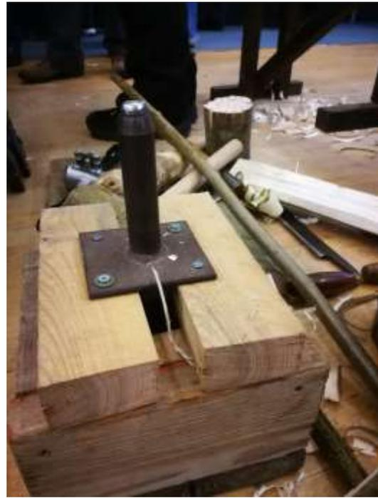
The next item was how to make the teeth on a rake. Using the Froe Ian split the log into small squares and then with a jig he turned them into rounded pins.
