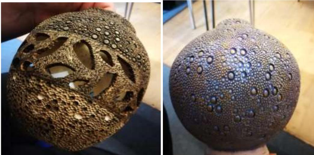
Ed repeated the process again using a piece of Ash. He marked up the centres and placed it between centres but this time he rounded it down with A Spindle Roughing gouge. He put a tenon on one end and shaped the piece with his long grind bowl gouge even though it was a spindle turning. If you wished you could burn the piece with a blow torch. (it's probably advisable to clear away any shavings) he the sprayed the piece with an airbrush.
