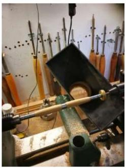
Next we come to the sanding. I start with 180 grit and go to 400; I mark the back of the abrasive with a number so it's easier to tell which grit is which. Don't forget to use your dust extractor.
