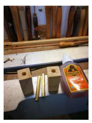
I glue in the tubes using Gorilla glue. You spray a little water down the hole in the blank, spread a little of the glue on the tube and insert it into the hole. The glue then foams up and ensures that any little holes are filled.
