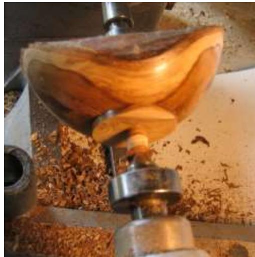
Outside sanded and polished and centre reduced to fit into chuck
