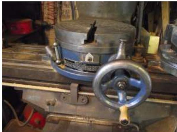
I centred this on my milling machine. I then moved the table 32.5mm to give me the radius for the holes, i.e. 65mm diameter. I then indexed the rotary table every 15° and centre drilled a small hole. When all the holes had been centred I drilled the 3mm holes on my pillar drill.
