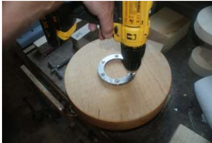
Screwing on an Axminster face plate ring.
