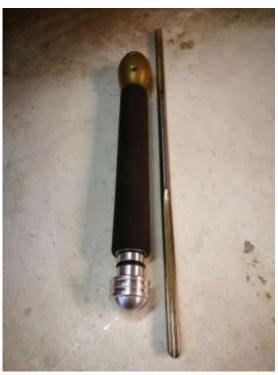
The silvery bit is the end of the handle with a built in Allen key to loosen or tighten the screws holding the tool. The theory is that you put it back in the handle and, therefore, you never lose the Allen key, but with the shaft of the tool pushed into the handle the end bit doesn't fit.
