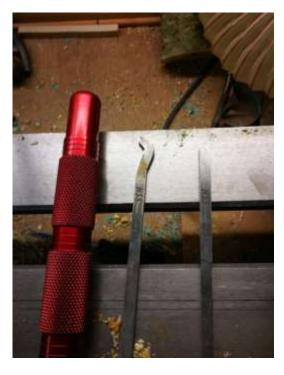
These, of course, cannot be sharpened on either the Pro-edge or any other mechanical sharpening system. I use a Diamond file as shown in the first picture using water as a lubricant. If you don't have water readily available you can use a little "Tongue Oil". (No it's not a spelling mistake it just sounded better than saying you can spit on the file).
