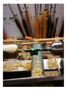
I start out by drilling a hole with an 8mm Brad point drill bit in the Jacob's chuck.
