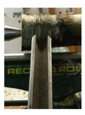
The shaping of the piece was done with a double ended Bowl gouge and handle as supplied by Hope Woodturning.
