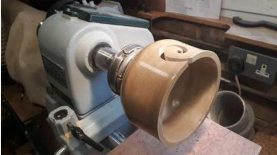
Using another lathe, where I can lock the headstock, I have made a template (attached to an old pillar drill post) so that I can utilise a router fitted with a 6mm cutter inside a 12mm guide. This sometimes works, but my main problem is I cannot see what is happening when making the cut.
