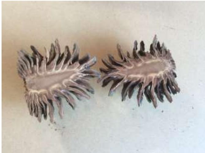
Pine cone cut through the centre and trimmed off at each end to fit the mould.
