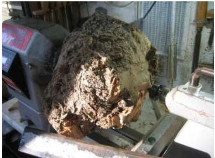
With the wood mounted between centres I set the lathe on its slowest speed of 100 rpm, stood well clear and switched on. Nothing disastrous happened so I increased the speed gradually to 350 rpm before vibration started to increase. Using my largest Bowl gouge I started removing the worst of the odd lumps but was cutting air for more than 90% of the time.
