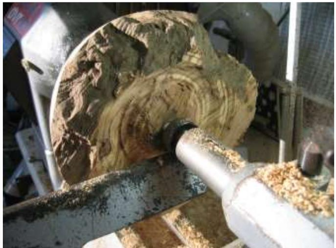
Hollowing continuing but tail stock is restricting cut so the tailstock was removed and headstock swivelled about 15 deg. to give better access without having to lean over the bed bars.
