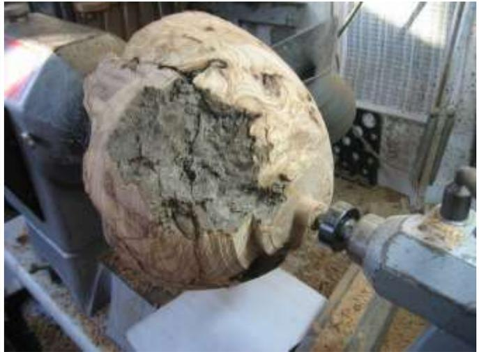
The piece was remounted into a chuck, but still with tail stock support, and hollowing started. I was continually edging up the speed and had now got to 800 rpm as some of the out of balance had been removed.
