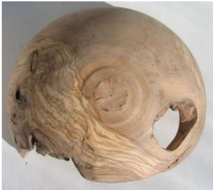
A piece of scrap wood was mounted in the chuck, slightly domed to match the bowl, and padded with a piece of router mat. With tailstock support the spigot was turned away leaving the bottom slightly dished and a small pip still under the revolving centre.
