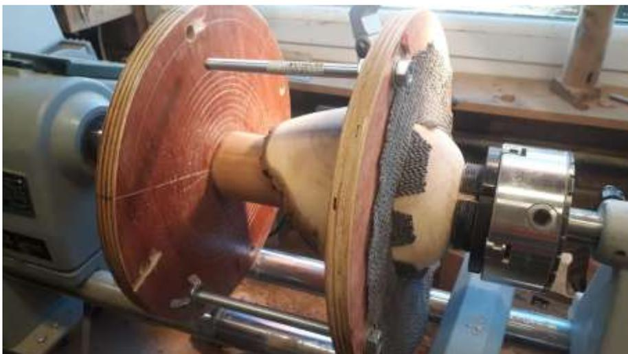
This allowed me to re centre the project into a slightly modified doughnut chuck. I turned a mushroom, which tenons into the doughnut to hold into the turned centre of the project. Once aligned in the doughnut the tailstock chuck was removed. Once the spigot was turned off, I was able to put whole thing into plastic sack, ready for my pals wood burning stove!
