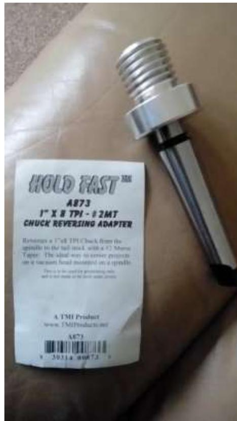
This is a centre that I use to hold a chuck in the tail stock. I recommend a slight encouragement with a wooden mallet to ensure a good grip. Although this centre has a 1 inch by 8 tpi thread, adapters to over threads could be used.
