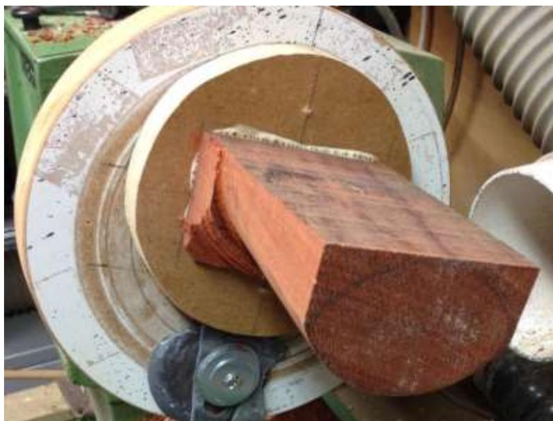
Now re fixed centrally on the faceplate to cut a slight shallow across the top and to hollow out.
