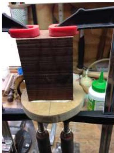
This is a MDF faceplate that has been used for something before; it has a recess cut in the other side to expand the jaws into. I have drawn a line through the centre to help with lining up.
