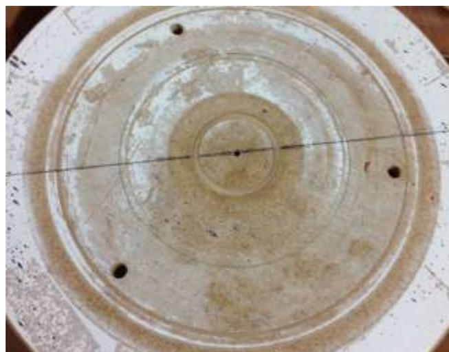
The sub base is fixed to the faceplate using the offset centre and the centre line.
