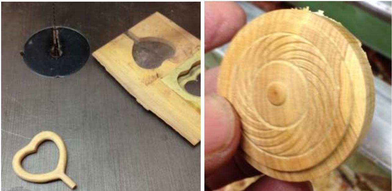
The lid is jam chucked and a 3mm hole drilled in the centre before shaping to a dome.
