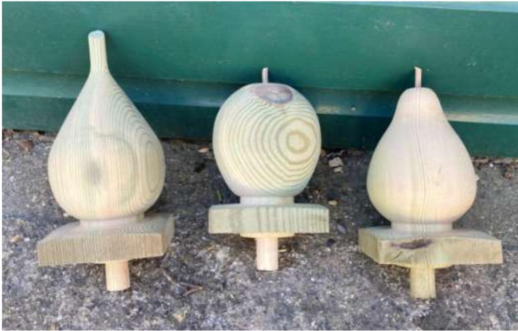
I wanted the bases to be kept square but then it's how to secure them to the top of the posts and then how to hold the blanks for turning. A bit of measuring followed and I decided thereabouts on a 25mm stem, 8mm deep chucking tenon, 25mm square section and then the fruit/veg shape. The initial shaping was to be done by holding the piece on a 4 prong drive and live centre in the tailstock.
