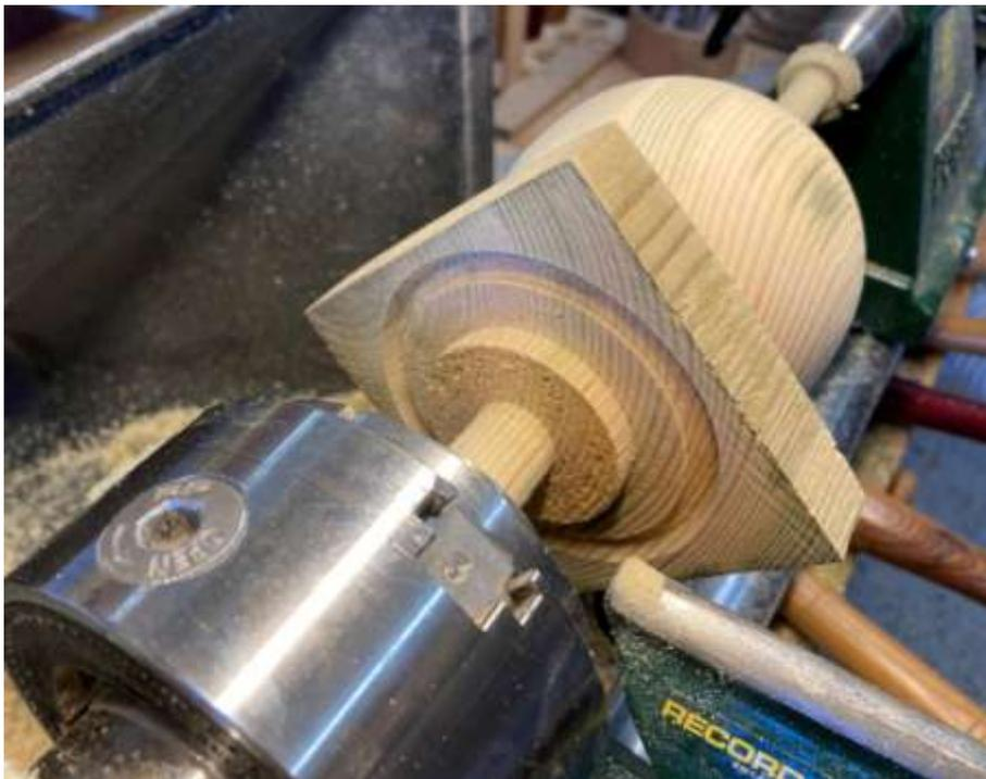
This I forgot to do which then involved remounting on the prong drive and associated hassle in getting things to run true etc. The drip groove can be simply cut using a suitable parting tool as there is no reason to cut anything fancy.
