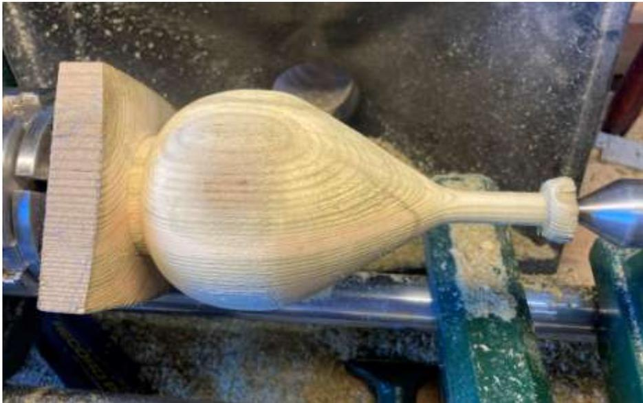
retaining the tail stock support until the last moment. When happy with your shape, sand to whatever grit you are happy with. As this is for outside and its pretty poor timber I just finished at 120 grit.
