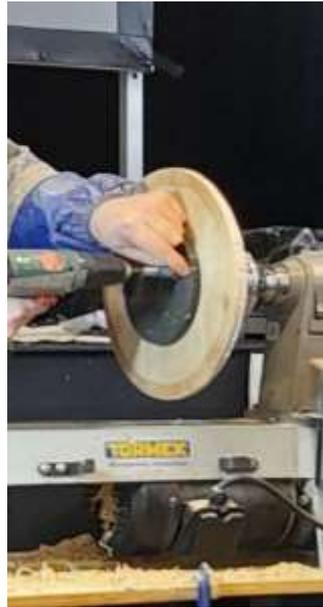
**HOT TIP:** Make a series of grooves in the timber no more than 1/2 mm deep as this will stop the gouge slipping.
