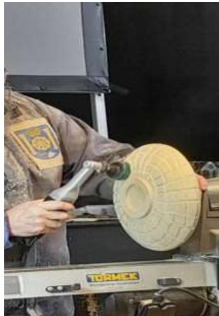
Using a long necked mini grinder with a Sabre tooth carbide cutter he textures the surface. He tends to go North, East, South and Westish. The Sabre tooth leaves rough edges so he uses an abrasive brush to smooth it all down. The brush is a Rolec M3.
