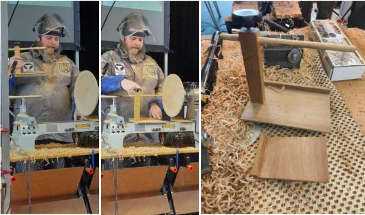
The base board is two parts the smaller part goes against the head stock and goes to the front of the jaws. It has a dowel which is aligned with the centre point. The gap between the two base boards is the depth of the bowl.
