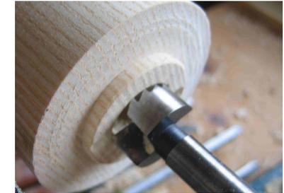
Pedestal to receive the base plate, 25 mm (1") bore for the nutmeg
