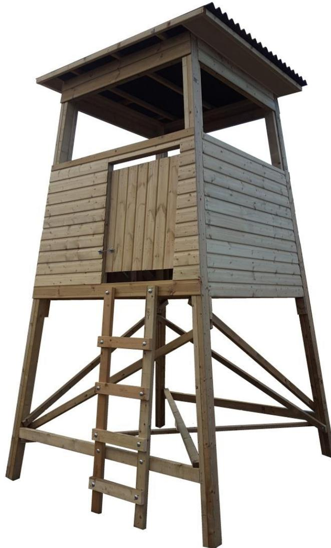
Free standing blind completed. For added security we recommend the 4 blind support legs are fixed down using 75mm (3") posts driven into the ground for 600mm and coach bolted or screwed through the posts into the framework.
