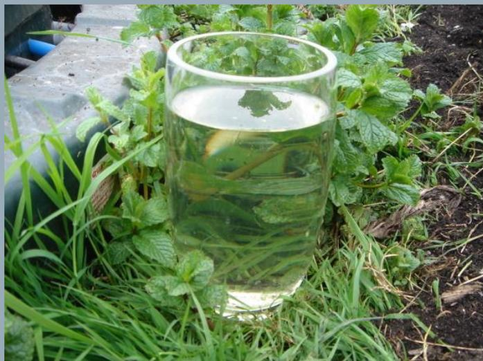
Effluent sample from a BioKube sewage treatment plant
