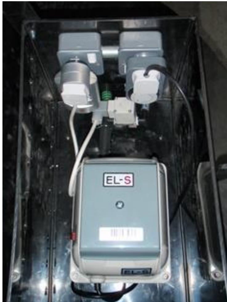
For larger Vortex units two air blowers are supplied and an additional socket will be needed.
