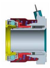
pressure to keep the bearing in contact with the clutch at all times. The CSC is more mechanically efficient than conventional cable or rod operated release systems.
