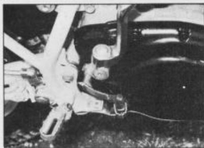
Rear brake lever (above) is shortened to protect it from rocks but makes brake less sensitive. 26mm carburettor (below) is set up for trials work with easily adjustable pilot screw with plastic cover and drain plug for float chamber.
