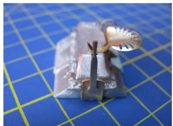
13, The brake lever can now be fixed to the rear of the cab as shown, the now completed gear box, seat etc can also be fixed in place. A small amount of white metal may require removing to allow access for the 8BA nut.
