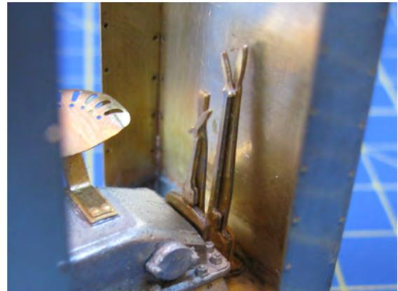
14, Using .45mm brass rod create hand rails at sides of cab.
