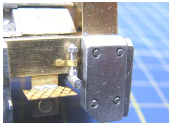
The starting handle can be fabricated using part 31 and a small length of .9mm and 1.5mm brass rod. Solder a 10mm length of .9mm brass rod to the slim side of part 30 and a 13mm length of 1.5mm brass rod to the wider side. Securing brackets can be made by using 2 x parts 30.
