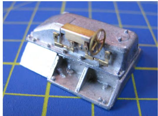
11, There are two etched hand levers included in the kit, the larger of the two (the brake) is situated at the rear of the cab. The lever situated slightly further forward and attached to the rear of the gearbox is the direction lever.
