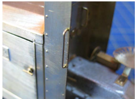
15, The white metal buffer plates, chassis weights, axle boxes and coupler pockets can now be fixed into place using adhesive. A dry run is recommended first to ensure all parts fit, a small amount of white metal may need removing from the rear of the chassis weights to make them sit flush with the buffer plates. Coupler pockets should be fixed centrally to the buffer plates.
