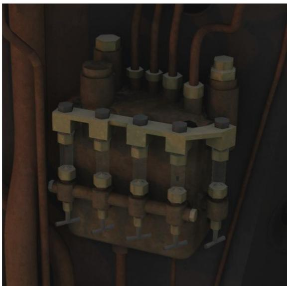
You can check that the jockey is open and the lubricator is working by looking at the drops of oil passing through the sight glasses of the lubricator. You can also adjust the speed of these oil drops using the sight glass valves – the ideal speed should be for a drop to pass approximately every 4 seconds.
