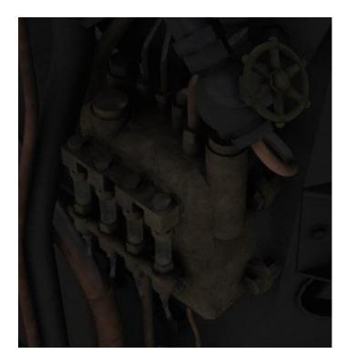
You can check that the jockey is open and the lubricator is working by looking at the drops of oil passing through the sight glasses of the lubricator. You can also adjust the speed of these oil drops using the sight glass valves – the ideal speed should be for a drop to pass approximately every 4 seconds.
