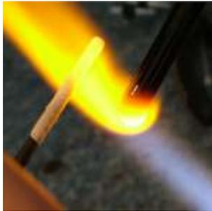
Heat a mandrel to a soft orange glow. This is important. If the mandrel isn't glowing orange then it's not warm enough. If the mandrel isn't warm enough when the hot glass comes into contact with it the glass will contract slightly and create tiny air bubbles in your bead.
