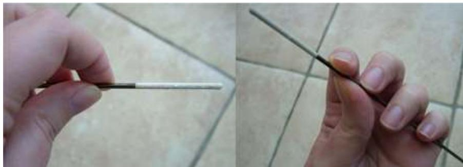
The picture on the left shows how I would hold the mandrel whilst making a bead and the one on the right is a view of what my fingertips are doing on the other side. The thumb and forefinger do the turning and the other three fingers steady the mandrel.
