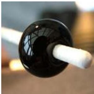
Once you're happy with your shape bring the bead out of the flame, keeping it horizontal, keeping it turning, and let the glow disappear completely. Then it's ready to place into a waiting warm kiln or into your fibre blanket or vermiculite.
