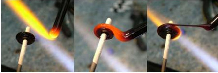
Let the glow come out of the tiny bead you've just made. If the bead is orange it means it's hot and the glass you've just applied will move and drag around with the next wrap that you're about to add.
