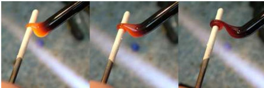
The key to neat bead holes (and by neat I'm referring to the nice 'dimpled' area around the holes as opposed to sharp pointy ends) is to make the initial the first wrap of glass much narrower than the desired width of the final bead. Here, my demo bead is going to end up at about 13mm diameter. My initial wrap is approximately 5mm diameter.
