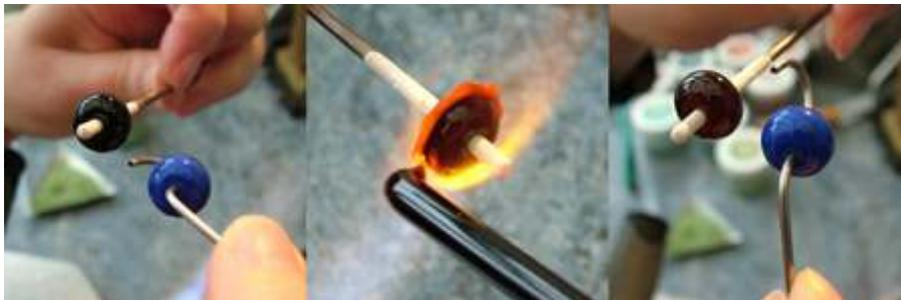
When I'm making a set of beads I choose what size I'd like the base of each one to be. I make the base bead by eye and when I've rounded it up I hold it up next to my chosen bead gauge. If I need more glass I add it around the centre of the bead, reheat, round up and measure again. Then I go ahead and decorate the bead, safe in the knowledge that size-wise my beads will more or less match. This is particularly useful when making earring pairs.
