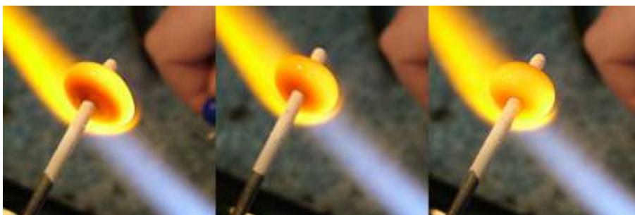
Now you need to put your bead back into the flame and heat it (while keeping that mandrel horizontal and turning slowly and steadily) to a nice even glow. The glass will start to move and the disc will condense down into a rounder bead. As it does this, the glass will start to slump over at the edges which is what creates the lovely dimpled bead holes that won't go on to cut beading wire and people's fingers.
