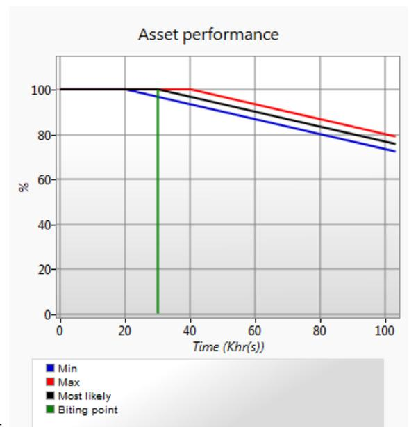
**Variability in all factors.** The catalysts very seldom perform in repeatable patterns, as some deteriorate faster than others. This can be put down to varying quality of the catalyst, environmental differences in the weather and seasonal patterns and feedstock variability in the process. To accommodate this variability, the minimum, most likely and maximum estimates were entered and illustrated here. Details of the costs estimates were entered in the study record.
