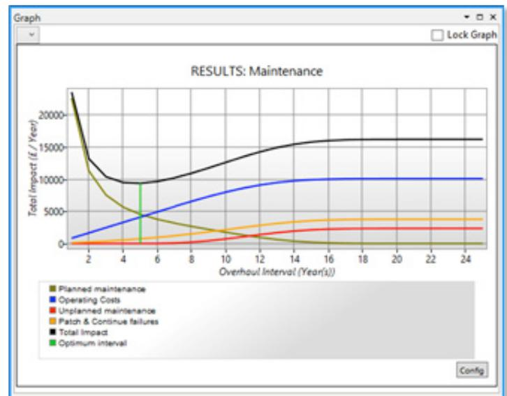
Figure 6: Optimum overhaul timing results
