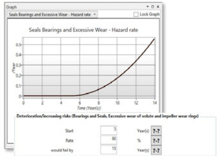
Figure 4: Unplanned maintenance failure pattern and hazard curve
