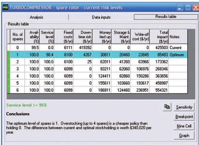
Figure 6. APT-SPARES evaluation of optimal spares requirements.
