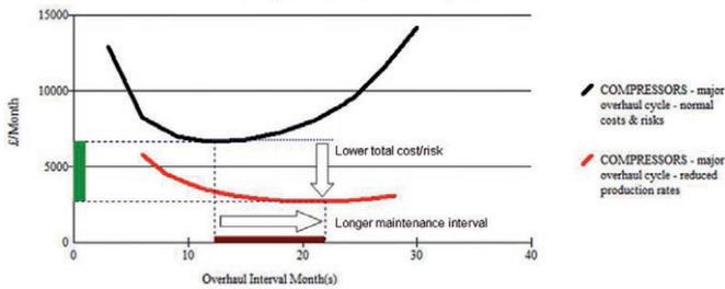
Figure 5. The impact of reduced production rates on maintenance intervals.
