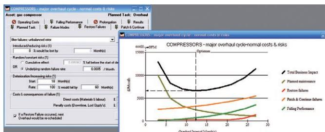
Figure 4. Calculating optimal maintenance intervals with incomplete data and structured tacit knowledge.
