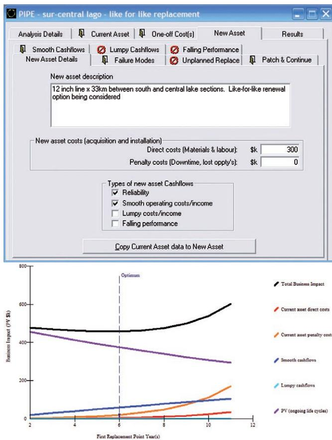
Figure 3. Optimal pipeline renewal timing.
