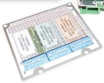
When used as a transformer TAP Position Transducer the operation is unique because it uses the actual switches as inputs instead of a resistance chain type which uses a resistance transmitter to convert resistance to say 4-20mA. The DSIT40 holds the output value between switching or if there is an invalid input. We can detect if a switch is faulty (i.e. more than one will be closed for an extended period of time).
