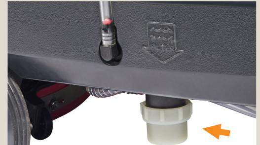
**Weekly:** Inspect the solution filter and clean if required.
