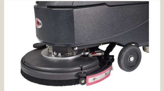
Place the brush or the pad-holder under the deck and Lower the deck or the brush/ pad holder by pressing the pedal. The squeegee is raised and lowered with the deck.
