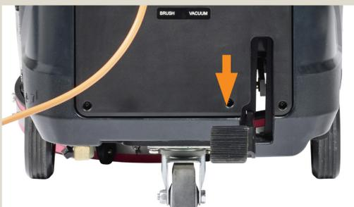
Lift the deck by pressing the pedal.
