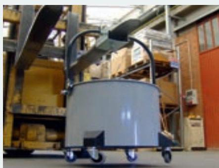
Container transport and discharge system with lift truck
