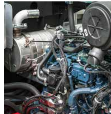
Tier 4/stage V ready engine with built-in diesel particle filter
