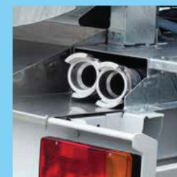
Handy storage space for suction hoses under the tank
