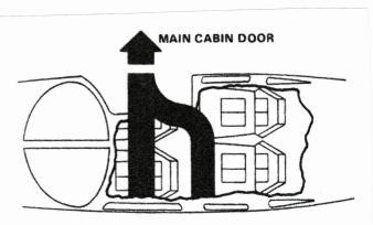
The seat backs of the front seats will push forward to ease the exit of passengers in the rear seats.
