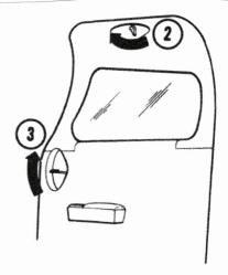
To open the main cabin door, twist the upper door latch (2) in a forward direction, and lift the lower latch (3) upwards. Then push door open.
