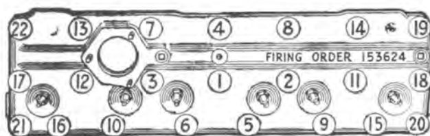
Fig. 7.—CYLINDER HEAD NUTS. Order for tightening.
